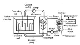
**Moderator:** In the fission of uranium, fast neutrons of energy 2 MeV are released. These fast neutrons have more tendency to escape instead of triggering another fission reaction. Also, slow neutrons are more efficient in inducing fission in  ${}^{235}_{95}U$  nuclei than fast neutrons. By the use of a moderator, the fast neutrons are slowed to thermal velocities. Usually, heavy water, graphite and beryllium oxide are used as moderators.
